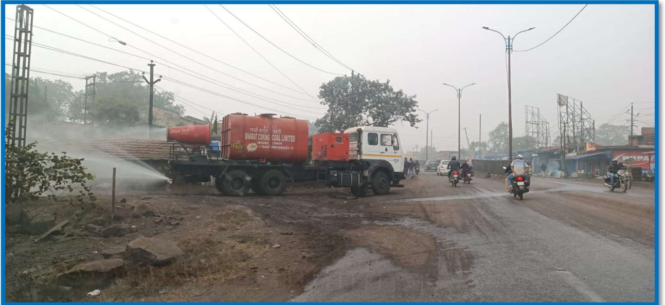
Picture 4 (II) – Truck Mounted fog canon on Transportation Road
